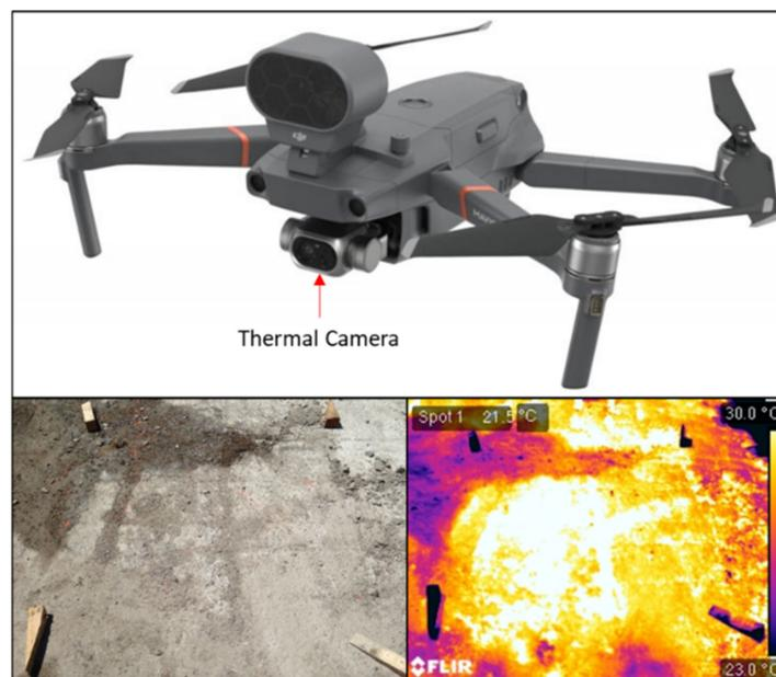
**Figure 7.** Typical IR-UAV equipment and sample thermography data.
