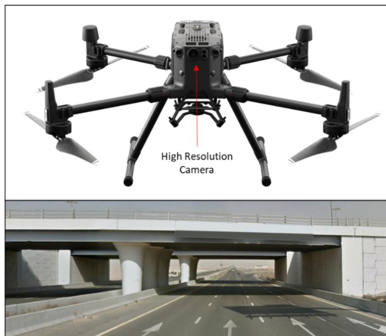
**Figure 6.** VI-UAV equipment and a sample of acquired data.
