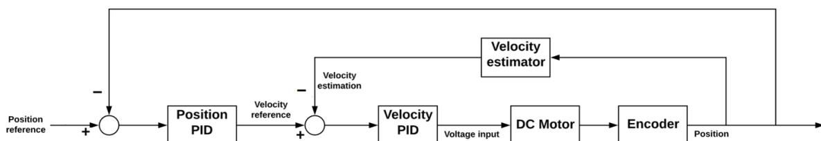
Figure 13. Feedback loop of position controller.
