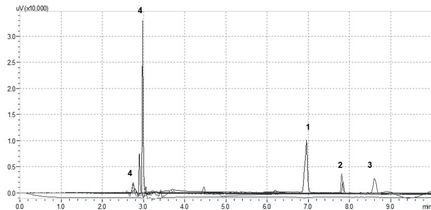
**Figure 2.** Selectivity of the HPLC-TBARS-EVSC assay. Chromatogram of 1: TBARS reaction (adduct); 2: sunscreen system and adhesive tape (irradiated and non-irradiated); 3: n-butanol; and 4: 0.2% BHT, H<sub>3</sub>PO<sub>4</sub> 0.44 M and 1% H<sub>2</sub>SO<sub>4</sub>. Retention time (min).
