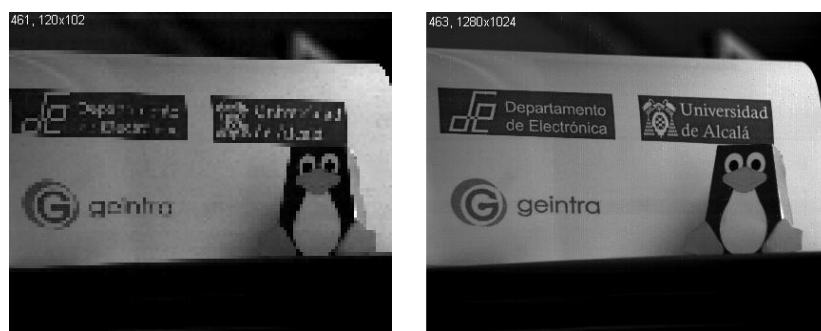
Figure 7. Captured and processed image from FPGA with different resolution. On the left, an 120 \times 102 pixel image and on the right, a 1,280 \times 1,024 pixel image.
