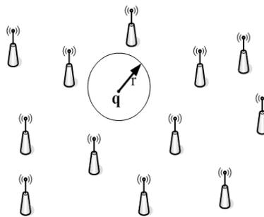
The area coverage shows the coverage condition of one wireless sensor network. Only under a certain area coverage, can a wireless sensor network work normally. To satisfy a prescribed area coverage  $f_a$ , the required intensity  $\lambda$  of the Poisson point process is  $\lambda = -\ln(1 - f_a) / \pi r^2$ . We can get the number of nodes to be placed in the sensing area from  $N(A) = \lambda * \|A\|$ .
