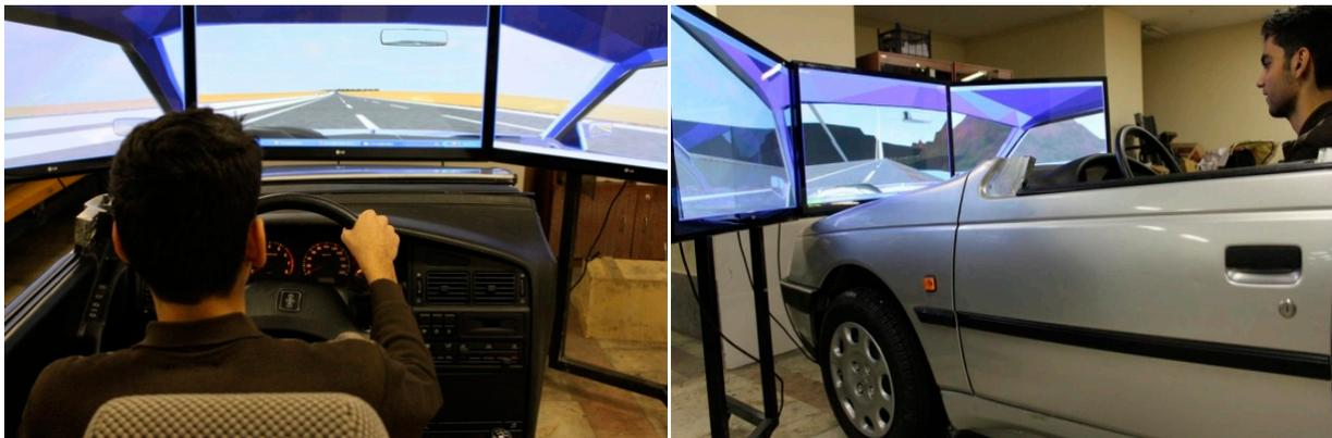
It is a fixed-base driving simulator with the active force feedback steering system and automatic transmission. Brake and gas pedals are equipped with the force and position sensors, respectively. The visualization system of the simulator uses three flat monitors and a sound system produces ambient and engine sounds. All communications and signal transmissions are carried out in real-time. The performance of the driving simulator has been already checked and validated [25].
