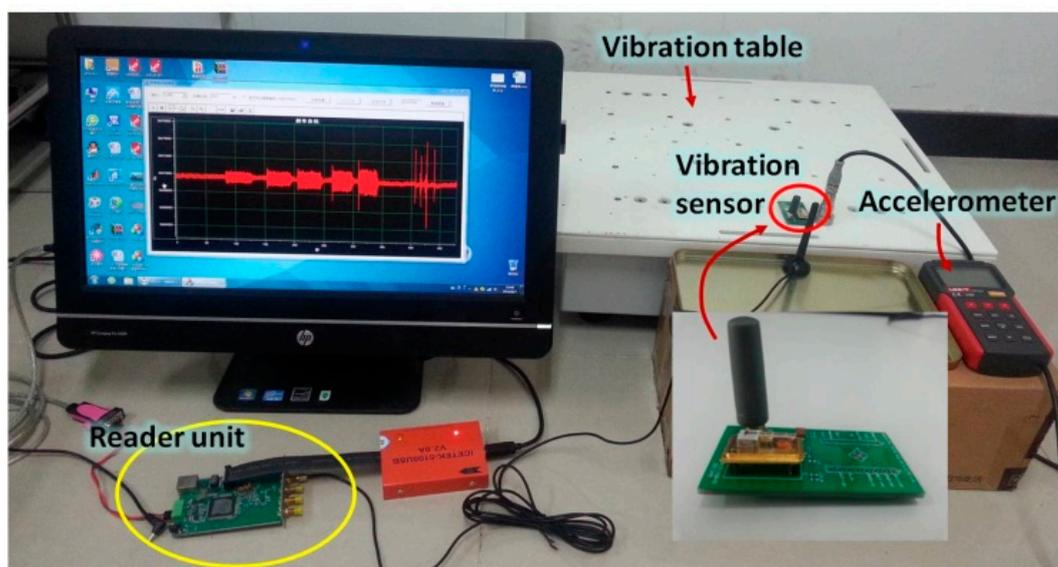
For wireless measurement, an interrogation unit (reader) utilizing the “frequency domain” method was employed (as shown in Figure 6), which interrogates a specific frequency with narrow-band pulse and then measures the returned signal power [17].
