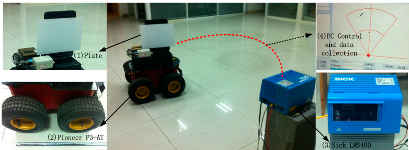
Figure 7. An overview of the proposed localization method based on a Laser Scanner. (1) The thin plate; (2) Pioneer P3-AT robot; (3) Sick LMS400 Laser Scanner; (4) Laptop software panel.
