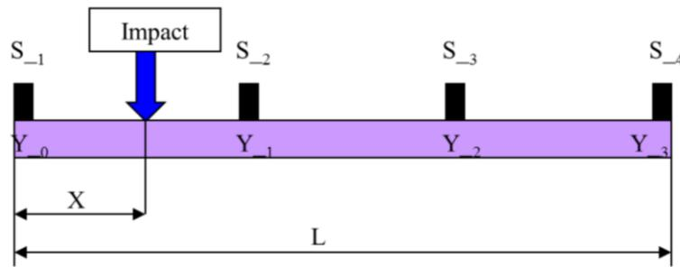
**Figure 2.** Mathematical modeling for an impact on a single bar with four piezoelectric sensors.
