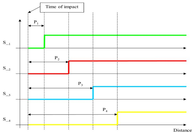
**Figure 3.** Time of impact on a single bar between sensors 1 and 2.
