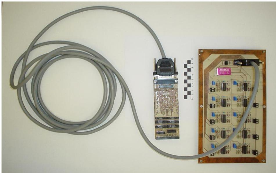
**Figure 5.** Electronic circuit for time delays measurements.
