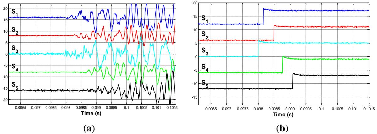
**Figure 9.** (a) Impact on  $P_2$ . Detailed view; (b) Edge signals when impacting on  $P_2$ .
