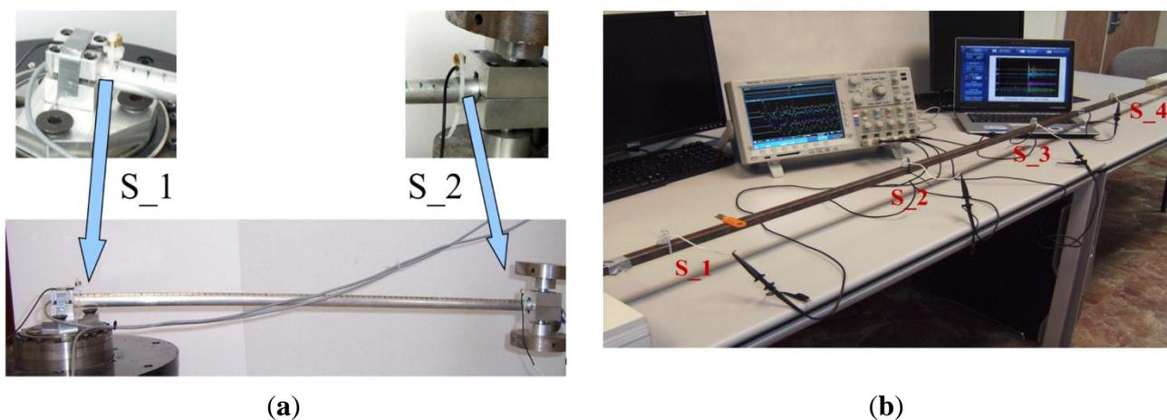
**Figure 1.** Experimental setup for an impact on a single bar with: (a) two piezoelectric sensors; (b) four piezoelectric sensors.
