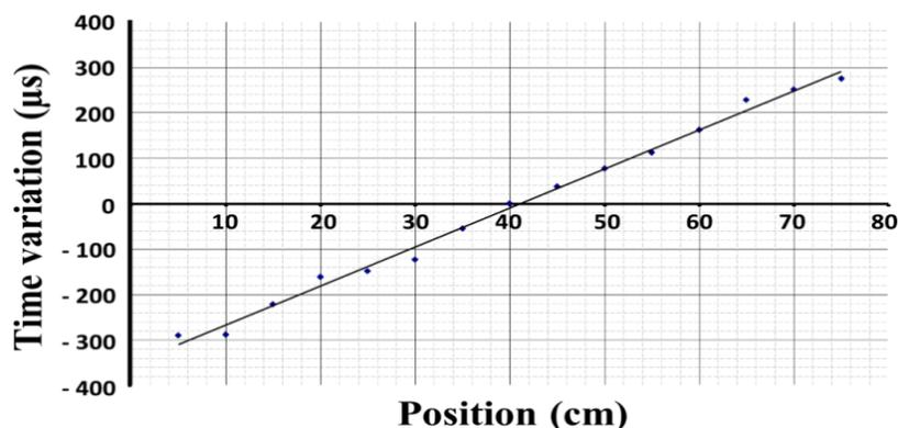
**Figure 6.** Calibration curve for an 80 cm bar.
