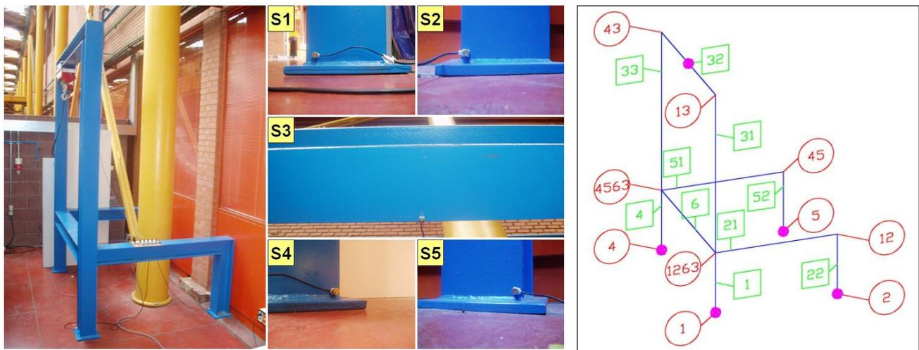
**Figure 7.** Geometrical description of the structure and sensors.
