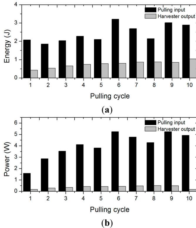
**Figure 9.** Mechanical pulling input and electrical output of all the cycles. (a) Energy; (b) Power.
