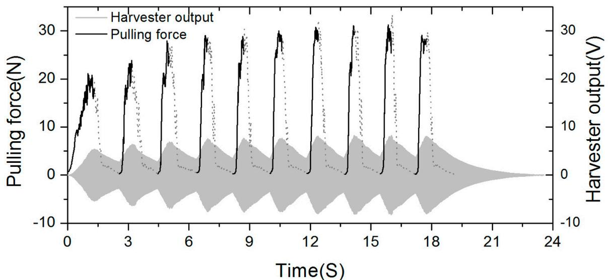
**Figure 8.** The recorded waveforms of pulling force and output voltage.
