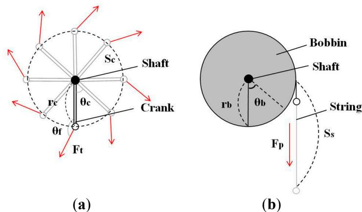
**Figure 2.** Analytic models of operation by human upper limb motion. (a) Turning; (b) Pulling.
