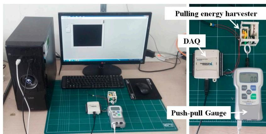
**Figure 7.** Experimental set-up for the simultaneous measurement of mechanical input and electric output power.
