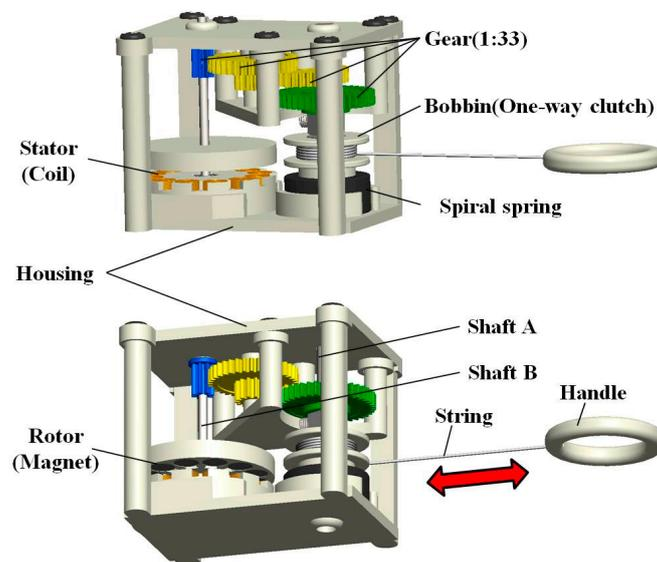
**Figure 4.** 3-D designed structure of the pulling energy harvester.
