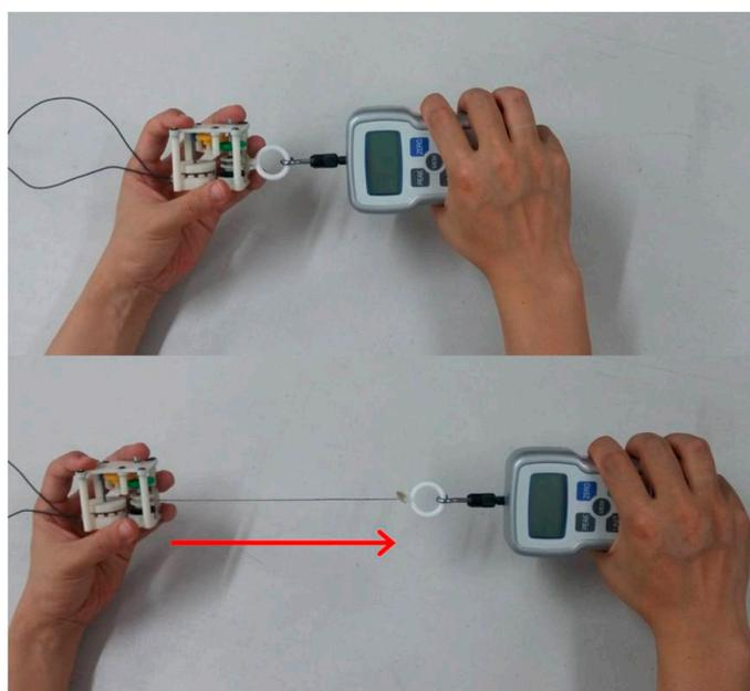
**Figure 6.** Pulling experiment using the developed prototype of pulling energy harvester and push-pull gauge.
