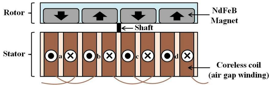
**Figure 3.** Electromagnetic coupling structure of the proposed APMM.
