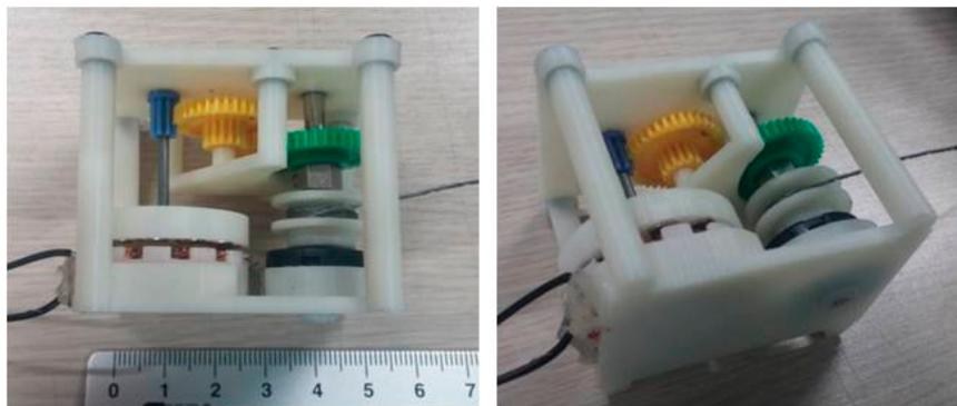
**Figure 5.** Prototype of the developed pulling energy harvester.
