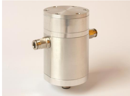
Figure 6. Assembled NDIR oil sensor prototype featuring 6 mm push-in hose connectors on either side and an electrical connector at the bottom of the sensor housing.
