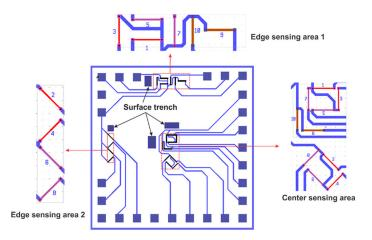
Figure 3. Chip layout out-of-plane shear stress and normal stress sensor developed on (111) wafer.
