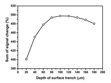
Figure 18. Effect of SCA depth on the percentage signal output sensing area 2.
