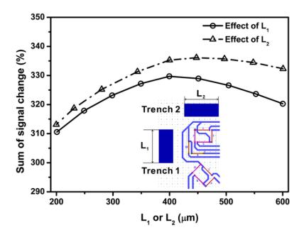
Figure 20. Effect of stress concentration area (SCA) length on the percentage signal output.
