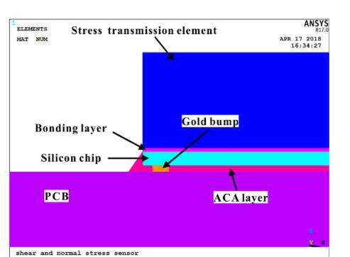
**Figure 5.** Schematic description of the FEM, including stress transmission element, bonding layer, silicon chip, ACA and PCB.
