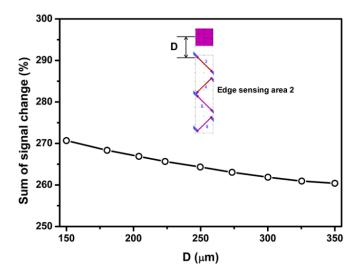
Figure 16. Effect of SCA depth on the percentage signal output sensing area 2.
