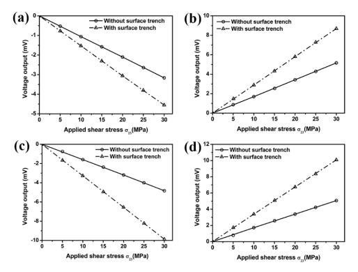
**Figure 10.** Effect of surface trench on the voltage output from resistors 1 (**a**), 3 (**b**), 5 (**c**) and 7 (**d**) located in edge sensing area 1.
