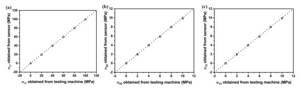
**Figure 26.** Comparison of out-of-plane normal stress  $\sigma_{33}$  (**a**) and shear stresses  $\sigma_{23}$  (**b**) and  $\sigma_{13}$  (**c**) measured from the sensor chip and the load cell of universal testing machine.
