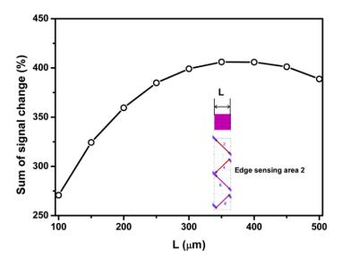
Figure 17. Effect of SCA depth on the percentage signal output sensing area 2.
