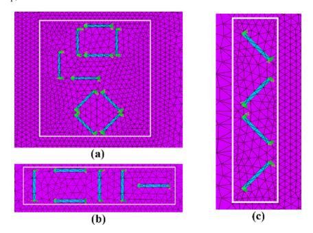
Figure 6. Mesh of the (a) center sensing area, (b) edge sensing area 1 and (c) edge sensing area 2.
