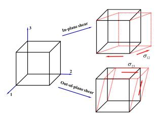
Figure 1. In-plane and out-of-plane shear stress.
