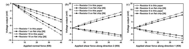
**Figure 27.** Comparison of signal output from the proposed sensor and the sensor in [22] for measuring out-of-plane normal stress  $\sigma_{33}$  (**a**) and shear stresses  $\sigma_{23}$  (**b**) and  $\sigma_{13}$  (**c**).
