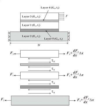
Figure 8. Force equilibrium diagram for five-layer analytical model.
