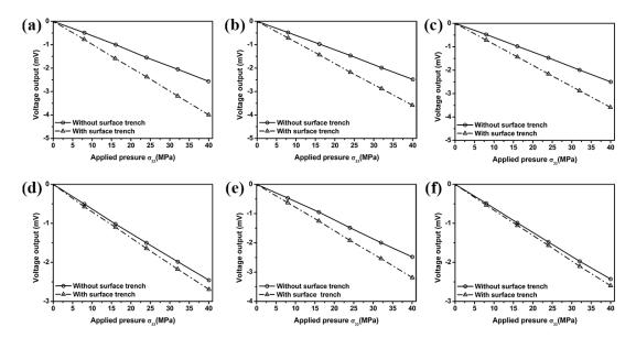
**Figure 12.** Effect of surface trench on the voltage output of resistors 1 (**a**), 3 (**b**), 5 (**c**), 7 (**d**), 9 (**e**) and 10 (**f**) located in the center sensing area.
