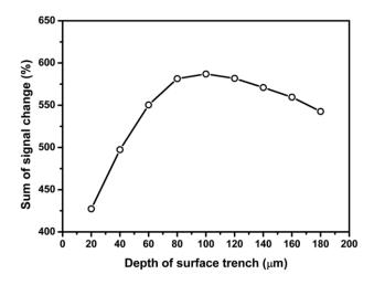
Figure 15. Effect of SCA depth on the percentage signal output sensing area 1.
