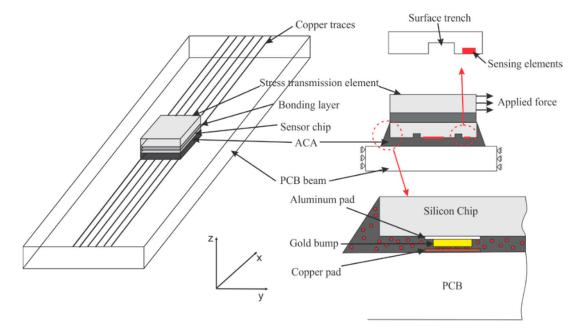
Figure 4. Schematic description of out-of-plane shear and normal stress sensor system.
