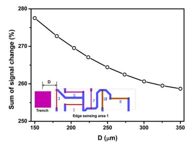
**Figure 13.** Effect of SCA locations (defined as the distance between surface trench and sensing area, D) on the percentage signal output.
