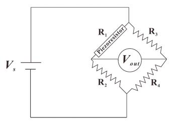
Figure 7. Wheatstone bridge configuration.
