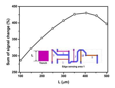
Figure 14. Effect of SCA depth on the percentage signal output sensing area 1.
