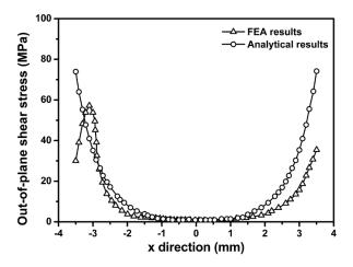
Figure 9. Out-of-plane shear stress distribution on silicon chip derived from analytical model and FEM.
