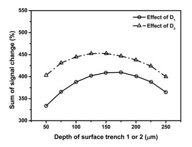
Figure 21. Effect of stress concentration area (SCA) on the percentage signal output.
