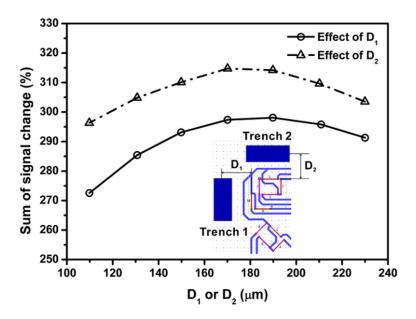
**Figure 19.** Effect SCA locations (expressed as D1 and D2, which are distances between stress concentration area and sensing elements) on the percentage signal output.
