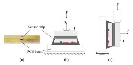
**Figure 24.** Assembled MEMS stress sensor on PCB beam (**a**) and schematic description of test setup for the measurement of out-of-plane normal stress  $\sigma_{33}$  (**b**) and out-of-plane shear stress  $\sigma_{13}$  (**c**).
