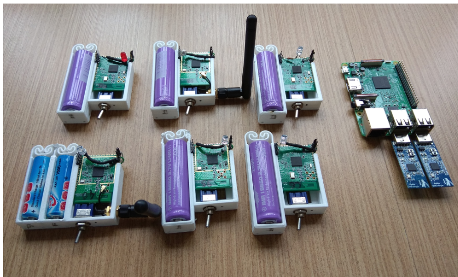
Figure 13. Test bed for the SD6WSN evaluation.
