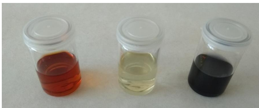
Figure S1. Steps to synthesize iridium nanoparticles ligand free. From left to right, red-brown solution from K_2IrCl_6 diluted in distilled water; yellow color due to the break of Ir-Cl bonds, creating the [Ir(OH)_6]^{2-} complex; and finally, deep blue obtained after the acid condensation, obtaining IrO_x nanoparticles ligand free.
