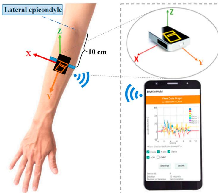
Figure 1. IMU placement.
