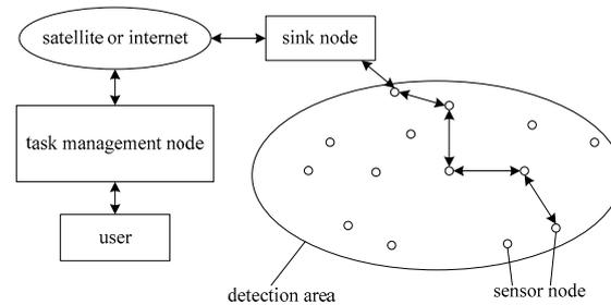
**Figure 1.** The architecture of WSNs.
