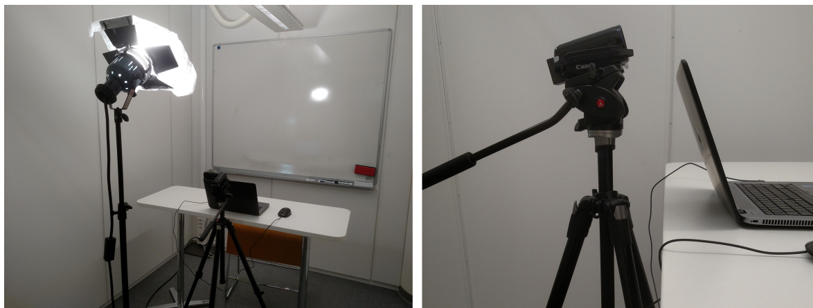
Figure 6. Experiment setup. On the left, an image illustrating the position of the equipment, including the angle of the external light source; on the right, an image highlighting the position and angle of the video camera.
