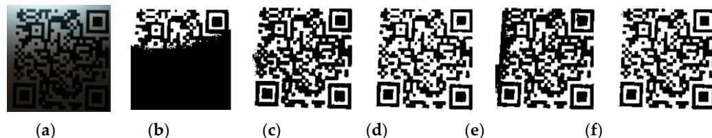
Figure 11. The original image and experimental results from different algorithms: (a) Original image; (b) Otsu's algorithm; (c) Niblack's algorithm; (d) Yao's algorithm; (e) Di's algorithm; (f) Proposed method.
