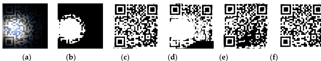
Figure 12. The original image and experimental results from different algorithms: (a) Original image; (b) Otsu's algorithm; (c) Niblack's algorithm; (d) Yao's algorithm; (e) Di's algorithm; (f) Proposed method.
