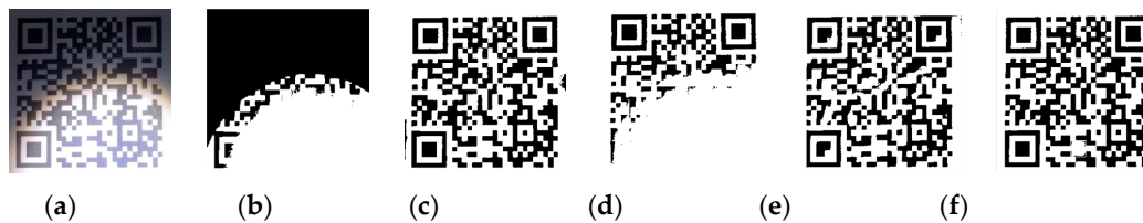
Figure 14. The original image and experimental results from different algorithms: (a) Original image; (b) Otsu's algorithm; (c) Niblack's algorithm; (d) Yao's algorithm; (e) Di's algorithm; (f) Proposed method.
