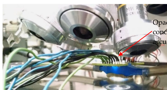
Figure 7. Measurement set-up: (a) generating soot for reproducible distribution; (b) window in the 3D-printed housing; (c) window under inspection during exposure.
