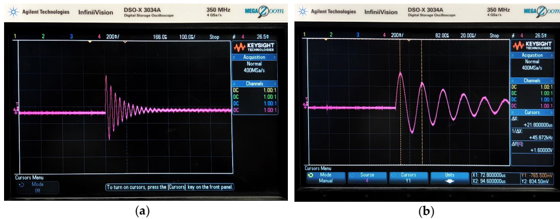
Figure 2. (a) Oscilloscope output for an undamped transient response of an RLC circuit where L = 64.3 \mu\text{H} and C = 0.2 \mu\text{F} with time on the x-axis and charge across the capacitor along the y-axis. (b) The cursors represent time period for the oscillation with the highest amplitude, the inverse of which gives us the resonance frequency.
