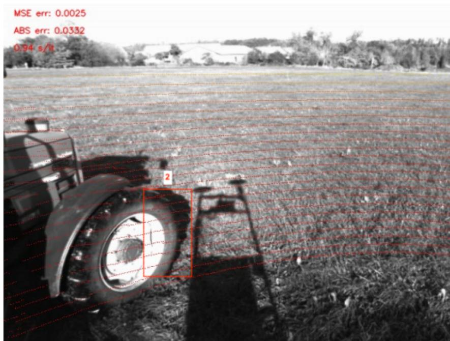
**Figure 6.** Example of LiDAR reprojected on the image. Note that a small error in the calibration will result in strong error on the estimated depth (see Square 2). We processed the error w.r.t. the depth obtained by stereo-vision.
