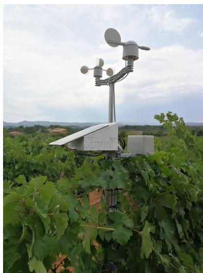
**Figure 8.** An example of *SEnviro* node deployed on a smallholding.
