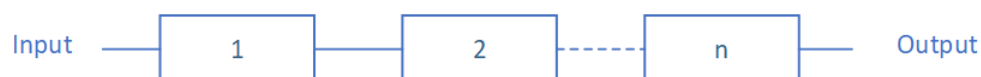
Figure 2. A series structure architecture according to the Reliability Block Diagram (RBD) paradigm.
