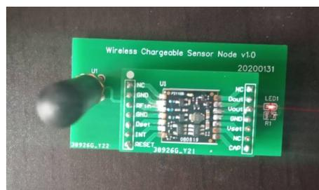
**Figure 4.** Practical experimental sensor node.
