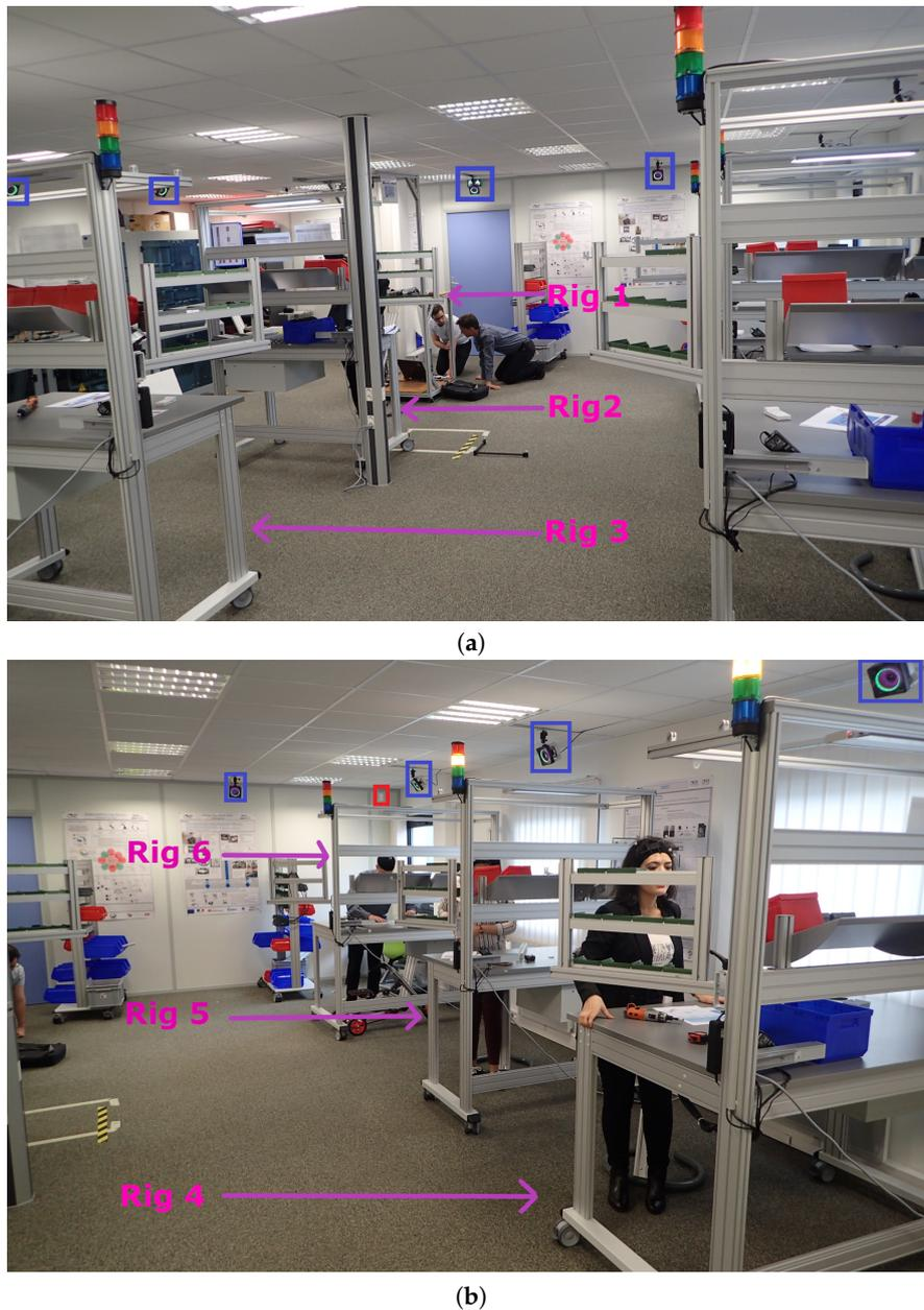
**Figure 2.** Our UWB set-up in an industrial NLOS assembly line. In the blue squares are the MoCap system and in red square the UWB system when not hidden due to NLOS conditions. (a) Industrial set-up in non-line-of-sight (NLOS) with six assembly rigs. view [A]. (b) Industrial set-up in NLOS with six assembly rigs. view [B].
