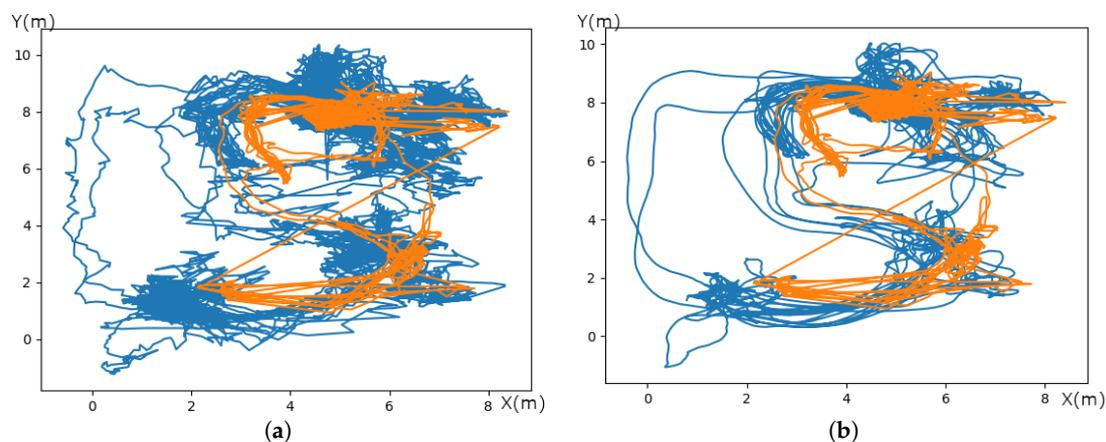
**Figure 12.** Comparison of the trajectory of the worker from station 1 between UWB filtered and not filtered in blue. In orange the motion capture system. (a) UWB system without Sav–Gol filter in blue and motion capture system in orange. (b) UWB system with Sav–Gol filter in blue and Motion capture system in orange.
