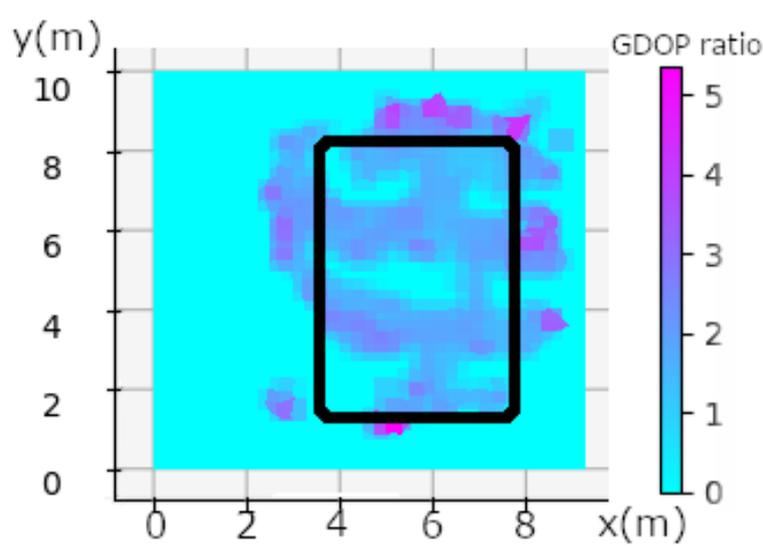
**Figure 9.** Geometric Dilution Of Precision calculation made in the workshop in the NLOS industrial condition. Black rectangles show the area where UWB anchors are placed, one of them in each corner.
