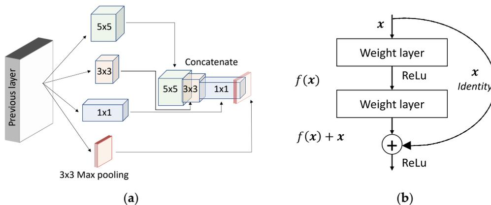
**Figure 5.** (a) The intuition behind the inception (V1) module in GoogLeNet. Screening local clusters with  $1 \times 1$  convolutional operations, screening spread-out clusters with  $3 \times 3$ , screening even more spread-out clusters with  $5 \times 5$  convolutional operations, and finally conceiving the inception module by concatenating (b) residual building block in ResNet.
