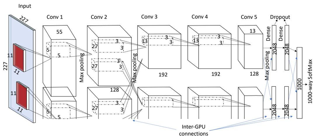
**Figure 4.** A typical architecture of AlexNet [14].
