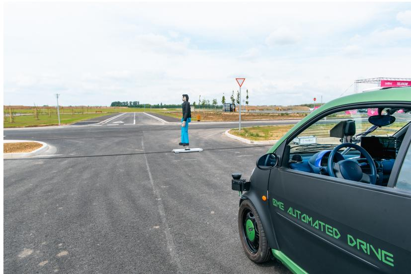
**Figure 4.** The VUT automatically stops while the 5G controlled dummy “walk” across the road.
