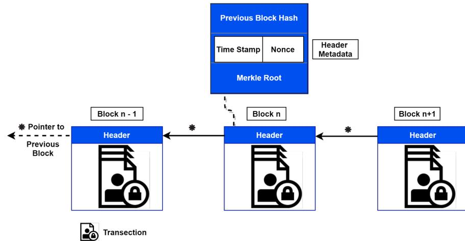
Figure 2. Composition of a block.
