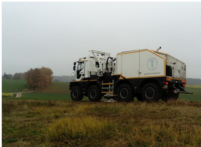
**Figure 3.** For the active part of the experiment a Vibroseis truck operated by the TU Bergakademie Freiberg (type: Thomas, VIB 3246) performed 480 sweeps.
