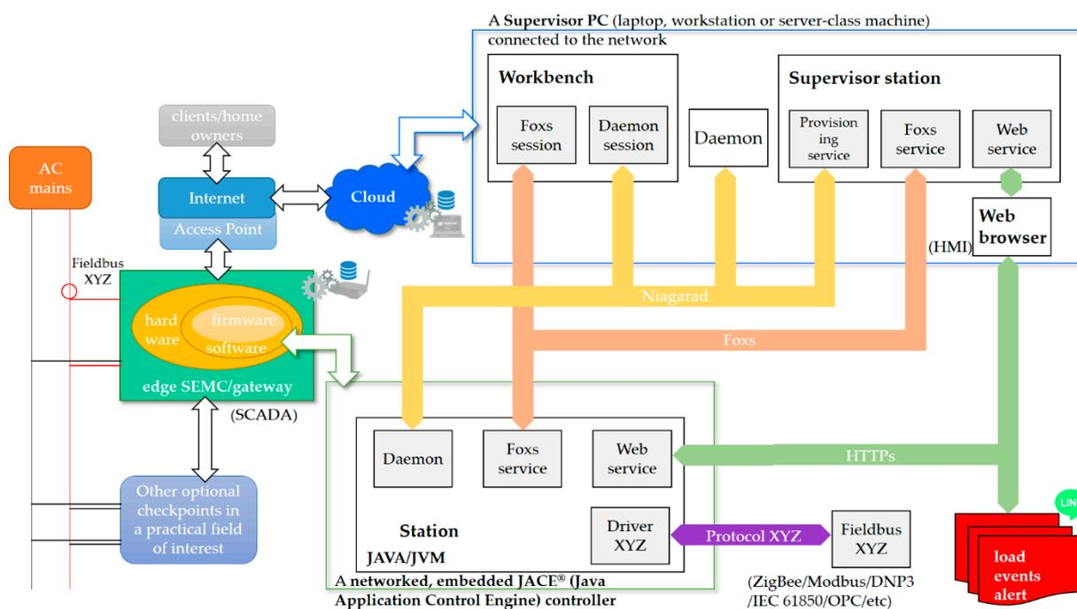
**Figure 4.** Configuration of the Niagara Framework® that considers a supervisor PC/laptop and a single-networked, embedded JACE® controller for SHEMS in this study.
