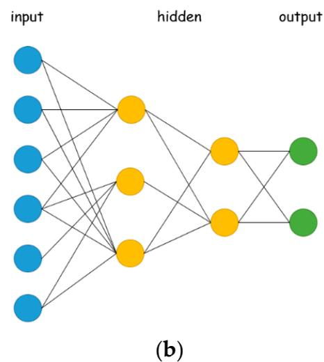
**Figure 7.** Representative artificial neural networks (ANNs): (a) An NN is fully connected; (b) An NN considers dropout—a hyperparameter whose value is specified and used to control the learning process of an NN—that can prevent overfitting [46] (another way used to prevent overfitting is early stopping).
