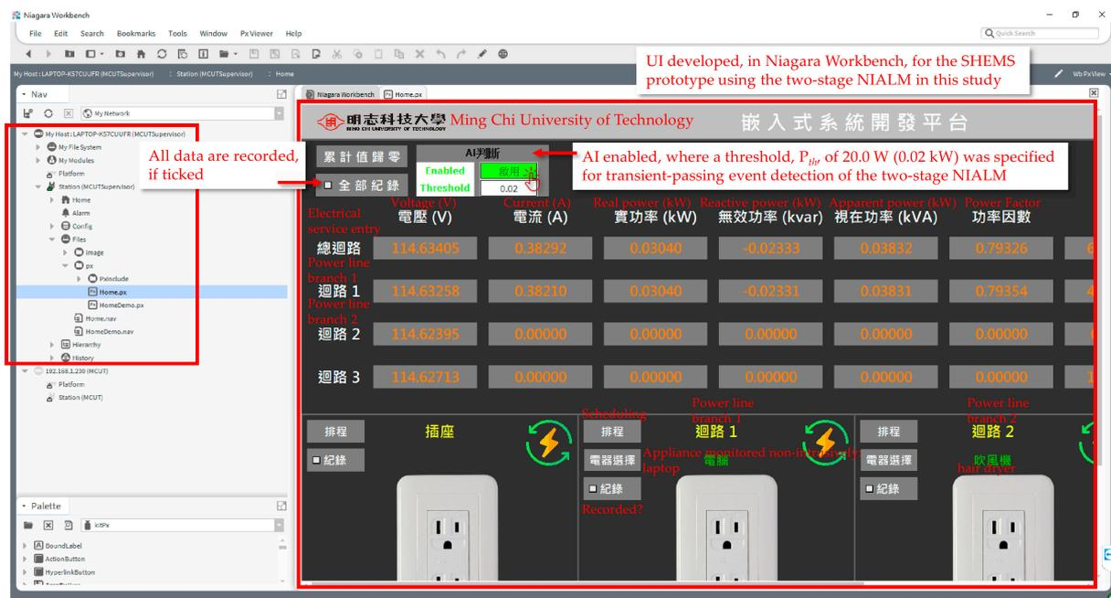
**Figure 11.** A user interface (UI) developed in Niagara Workbench for the established SHEMS prototype using the presented two-stage NIALM over fog-cloud computing in this study.
