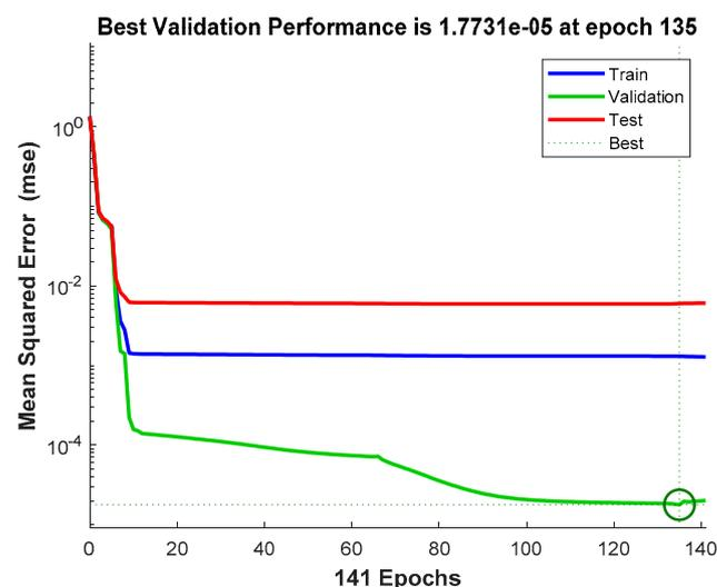
**Figure 9.** Training trajectory of the developed feed-forward, multi-layer ANN in this experiment, where the training process terminates at the 141-th epoch.
