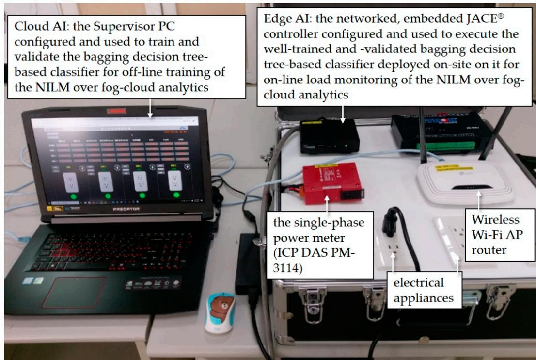
**Figure 8.** Experimental setup of the developed SHEMS prototype utilizing the presented two-stage NIALM approach over fog-cloud computing for the purpose of residential DSM. An electrical network topology with four power line branches in parallel is also shown.
