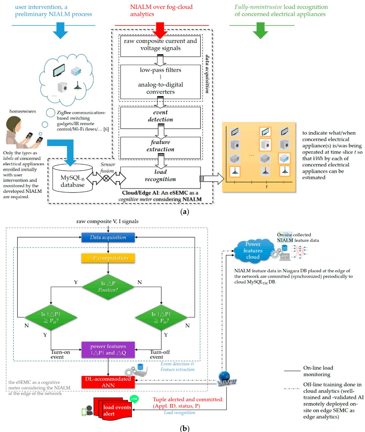
**Figure 5.** Investigation of the presented NIALM approach: (a) Pipeline of the two-stage NIALM, in simple terms, not requiring a one-time intrusive period for the preliminary NIALM process [6]; (b) the two-stage NIALM, based on the Niagara Framework<sup>®</sup>, over fog-cloud computing.
