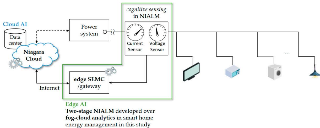
**Figure 2.** Developed NIALM approach over fog-cloud computing for smart home energy management in this study. Edge SEMC refers to the smart energy management controller considering edge computing.
