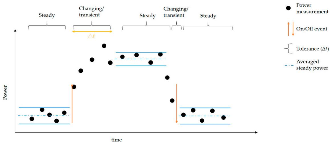
**Figure 6.** Detecting an appliance event in acquired total energy consumption through transient-passing event detection.
