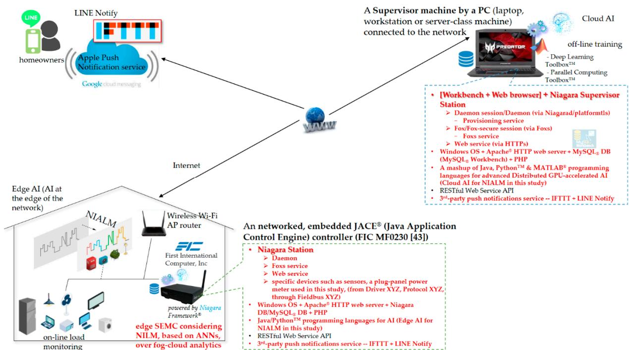
**Figure 3.** Developed smart home energy management system (SHEMS) prototype considering new two-stage NIALM over fog-cloud computing in this study, where the prototype is based on Tridium’s Niagara Framework®. The framework runtime is targeted for Java 8 SE compact3 profile compliant virtual machines (VMs). MATLAB® is suited and used as the cloud here.
