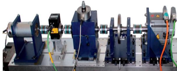
**Figure 6.** PU data testbed: test motor, measuring shaft, bearing module, flywheel, load motor (from left to right) [1].
