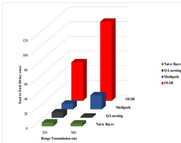
Figure 12. End to End delay vs. Range transmission.
