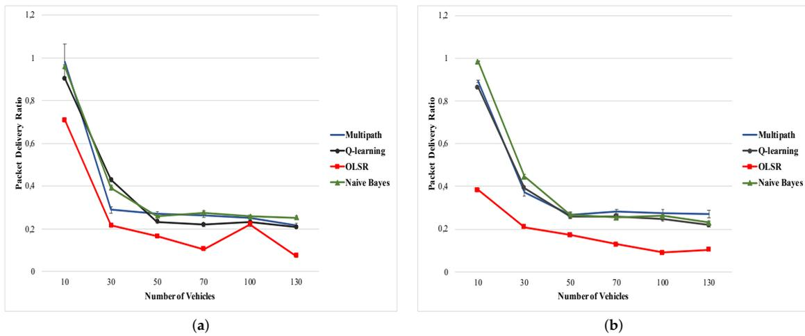
Figure 7. Packet Delivery Ratio vs. number of vehicles (a) range 250 m, (b) range 500 m.
