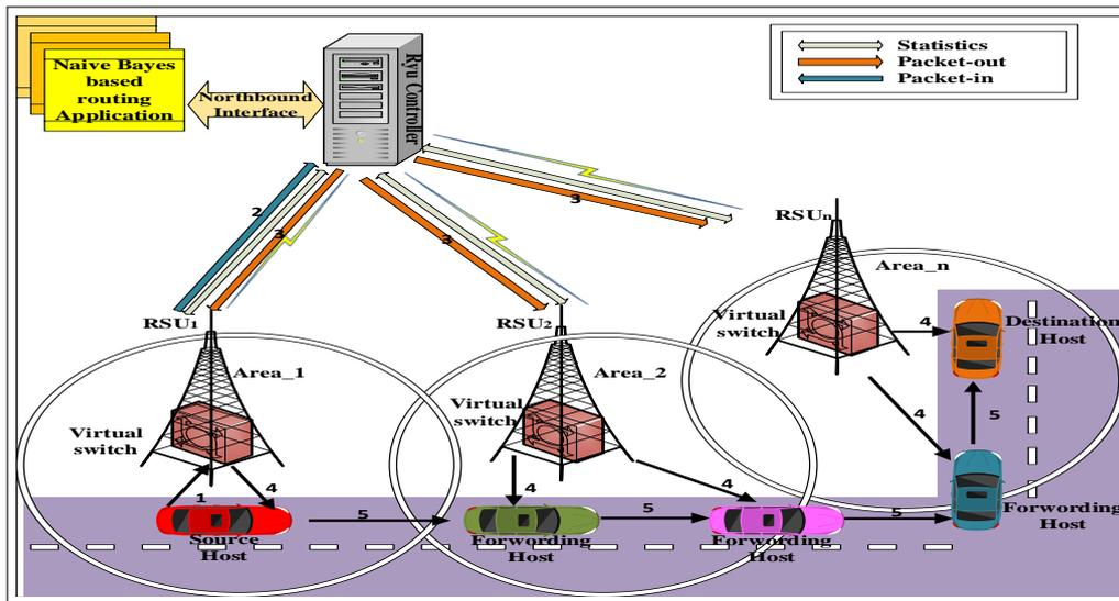
Figure 6. SDN-Naive Bayes-based Routing Protocol Operation.
