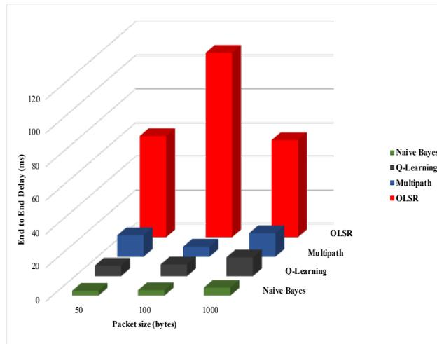
Figure 11. End to End delay vs. Packet size.
