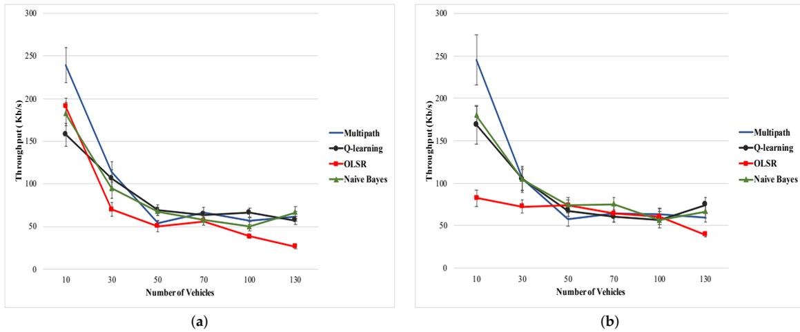
Figure 9. Throughput vs. number of vehicles (a) range 250 m, (b) range 500 m.
