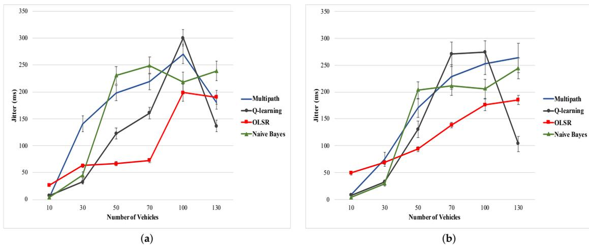
Figure 10. Packet Jitter Derivation (Jitter) vs. number of vehicles (a) range 250 m, (b) range 500 m.
