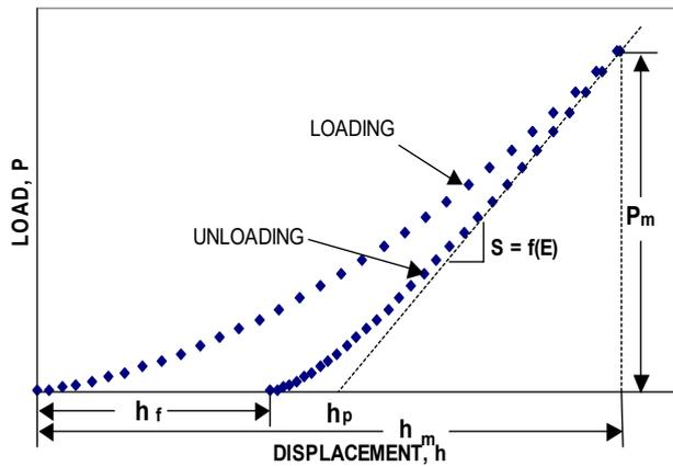
**Figure S1.** Schematic illustration of the thin film mechanical property measurement by nanoindentation.
