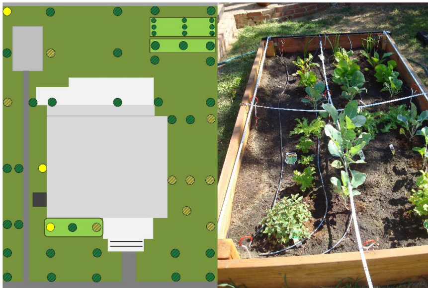
Figure 1. An example of a sampling map that is shared with study participants (left). The circles represent where the soil was tested for lead and the colors correspond to different lead levels. A raised-bed garden that was sampled for soil lead is shown on the right.
