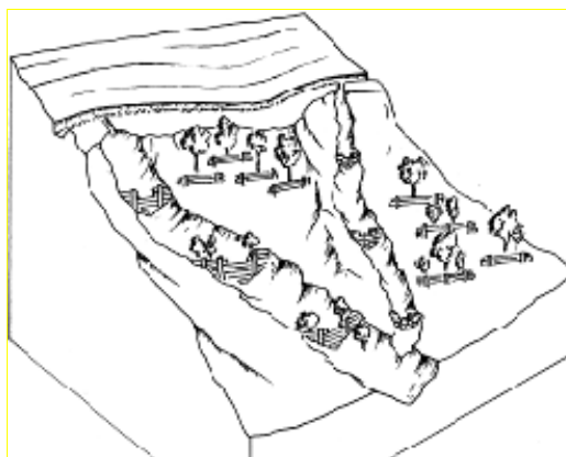
Gully control and catchment protection with integrated measures such as cut-off drains, wooden check dams, stone check dams and staggered structures for tree planting. Cochabamba, Bolivia. (Drawing: Mats Gurtner)
