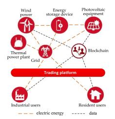
Figure 8. Blockchain-based power trading process [48].
