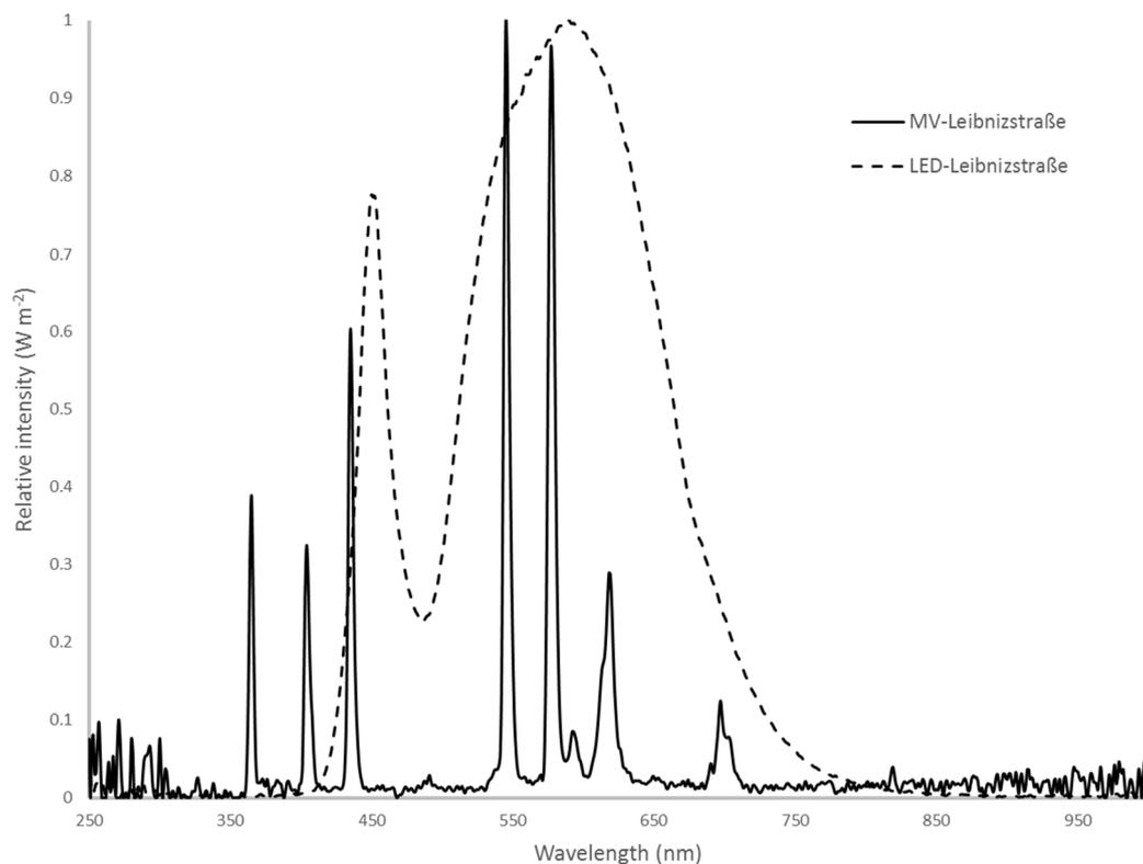
**Figure 1.** Spectral composition of both light sources used in Leibnizstraße - LED and mercury-vapor - as an example for different spectral compositions at a similar correlated color temperature (neutral white light around 4000 K). Graphs are standardized to a peak of 1.
