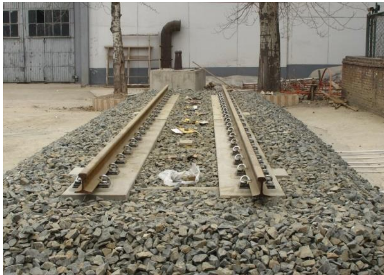
Figure 4. The ballasted ladder tracks in the laboratory.
