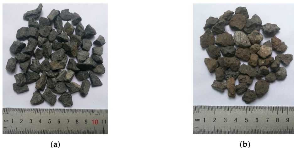
Figure 1. Appearance of 100 g of coarse aggregate: (a) basalt coarse aggregate (BCA); (b) steel slag coarse aggregate (SSCA).
