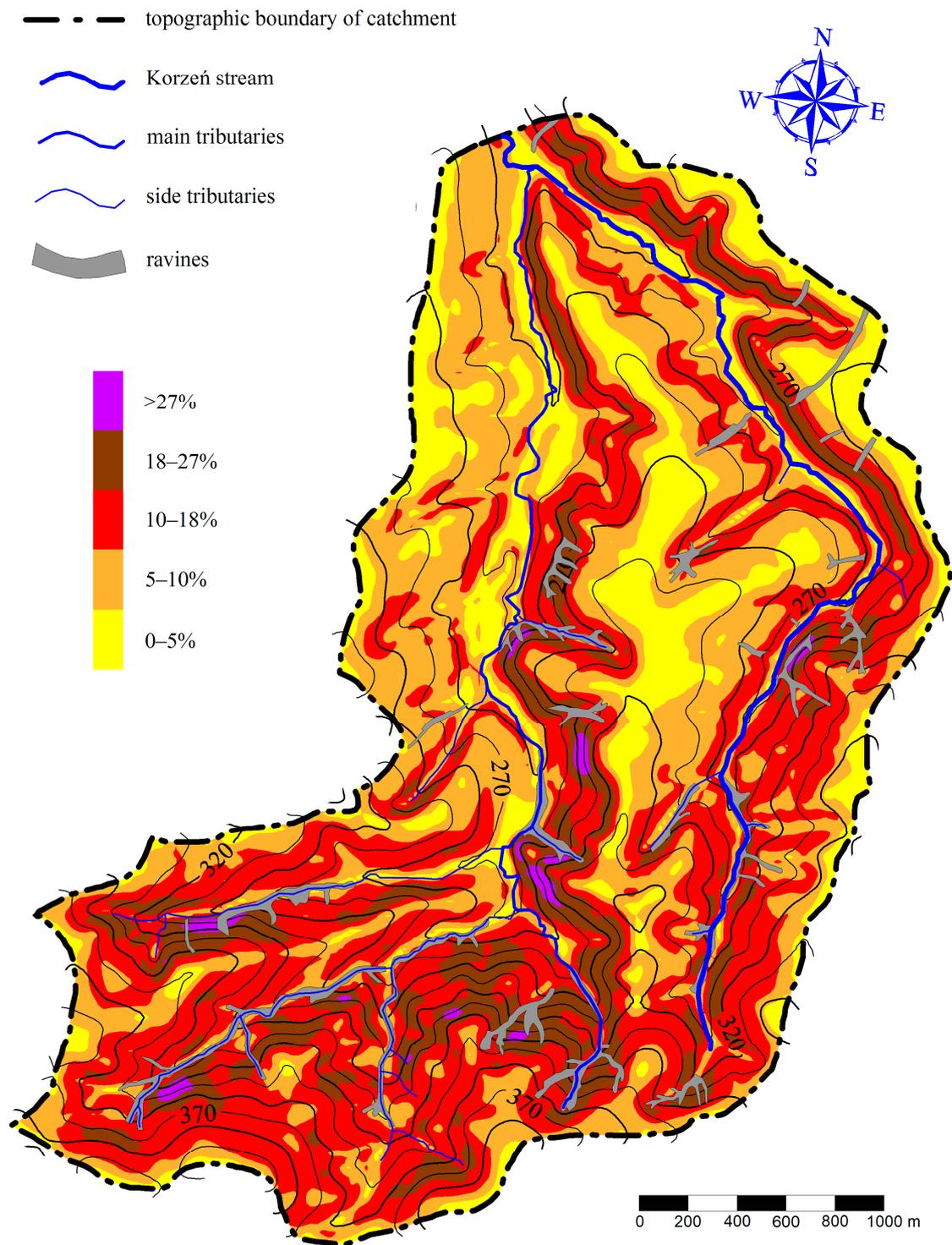
**Figure 2.** Slope steepness map of flysh stream in catchment area.
