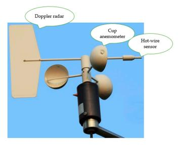
**Figure 4.** Cup and hot-wire, hybrid anemometer, Reprinted from Francisca et al. [40] with permission under the terms of the Creative Commons Attribution License. http://creativecommons.org/licenses/by/4.0.
