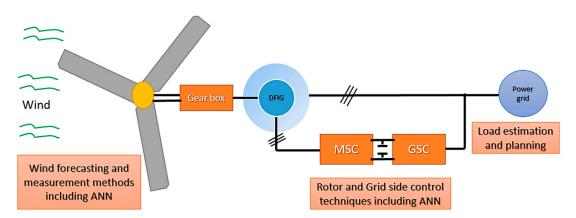
**Figure 8.** Illustration of the atmospheric effects on the wind-based doubly fed induction generator, producing energy and related control schemes for a sustainable system.
