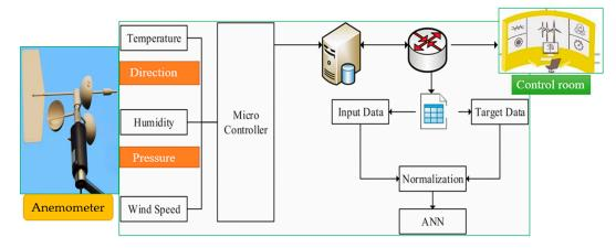
Figure 6. Wind power forecasting system.
