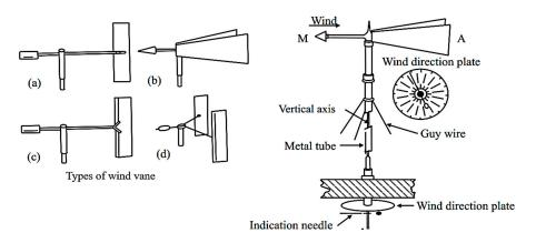
Figure 5. Wind vane and its types.
