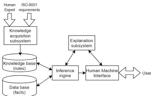
Figure 5. System architecture.
