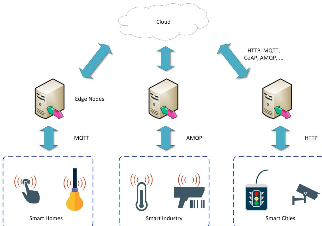
**Figure 1.** Edge Computing architecture, based on the work of Yu et al. [30].
