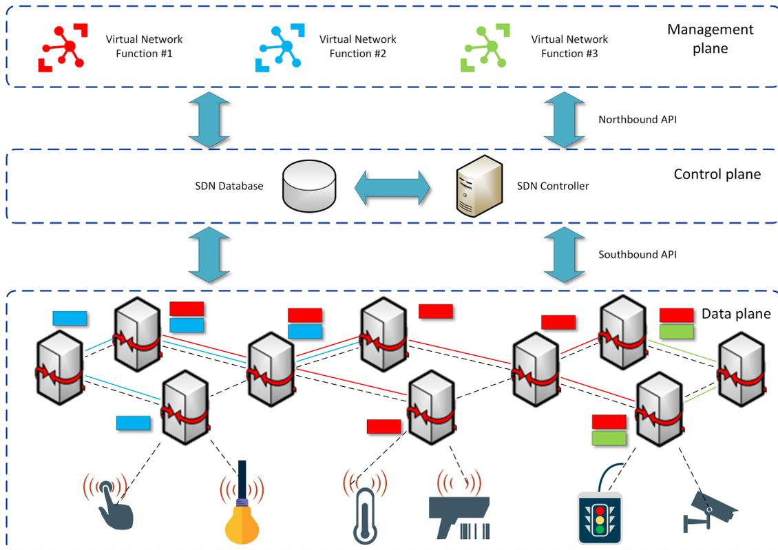
Figure 3. Network Function Virtualization (NFV) over Software-Defined Networks.
