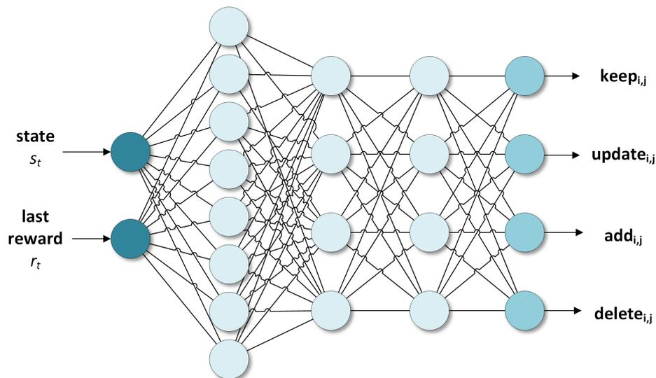
**Figure 6.** Q-Network used in Global Edge Computing Architecture (GECA) 2.0 SDN mechanism.
