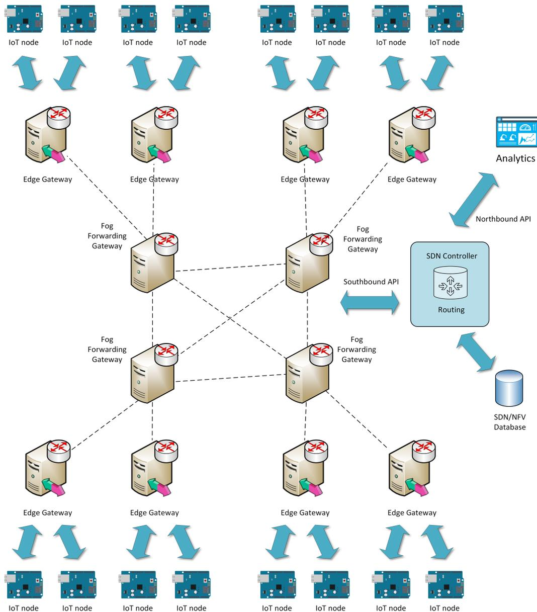
**Figure 7.** Emulated Fog-Edge-Internet of Things (IoT) network used for the experiment.
