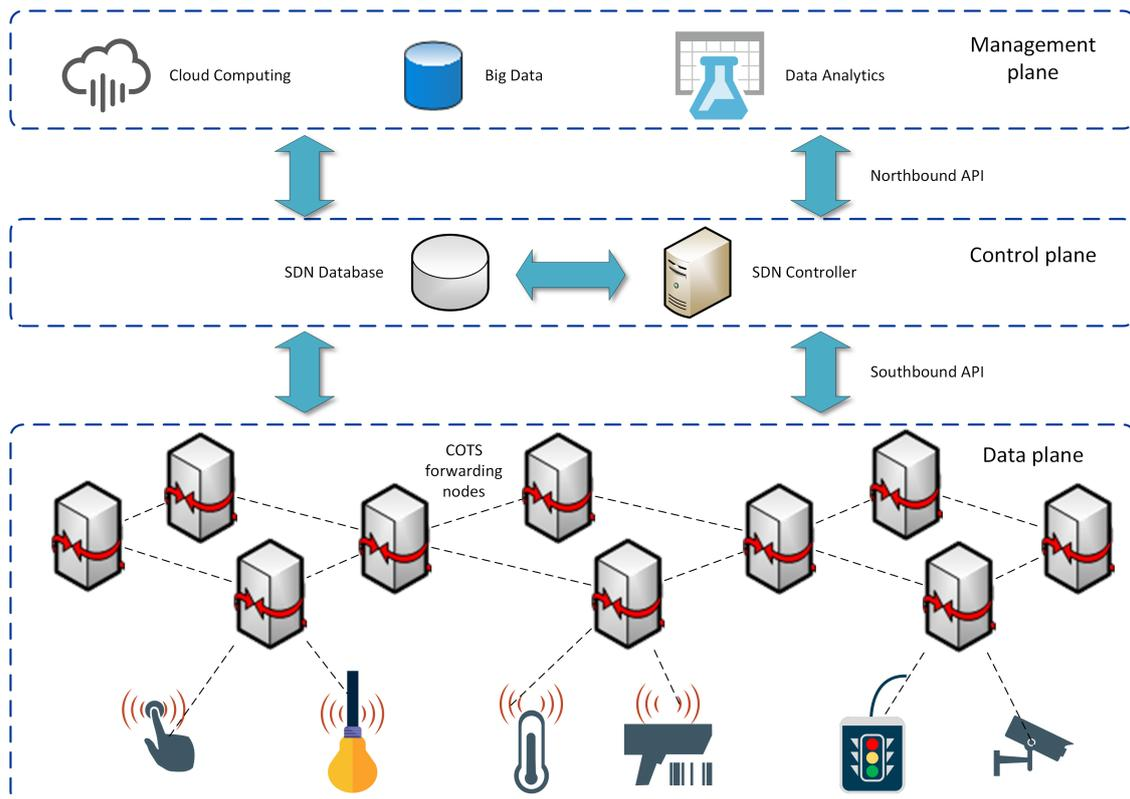
Figure 2. Software Defined Network (SDN) architecture.
