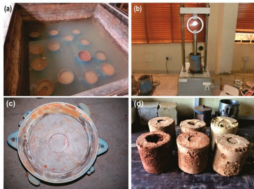
Figure 2. (a) Soaking of natural soil and lime-lateritic soil samples (b) Experimental device for determination of CBR values of natural soil and lime-lateritic soil samples (c) Standard mould used for the CBR test and (d) lime-lateritic soil samples extruded from the mould after CBR test.
