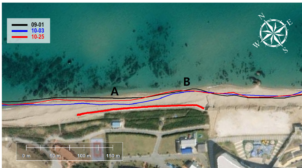
Figure 9. Shoreline positions marked on a Google Earth map. The thick solid red line marked inland denotes the location of the revetment. The thinner colored lines denote the shorelines calculated by the VMS on 1 September (black), 3 October (blue), and 25 October (red).
