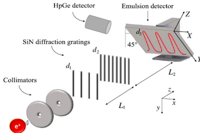
**Figure 2.** Scheme of the QUPLAS-0 detector experimental configuration. The collimated positron beam propagates through the interferometer, consisting of two gratings and the emulsion detector (tilted by  $45^\circ$ , see text). The interference pattern is collected in the emulsion. A Ge detector is used to monitor the positron beamline through the 511-keV gammas generated by positron annihilation.
