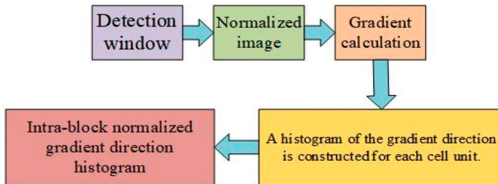
Figure 1. Histogram of oriented gradient (HOG) feature implementation process.
