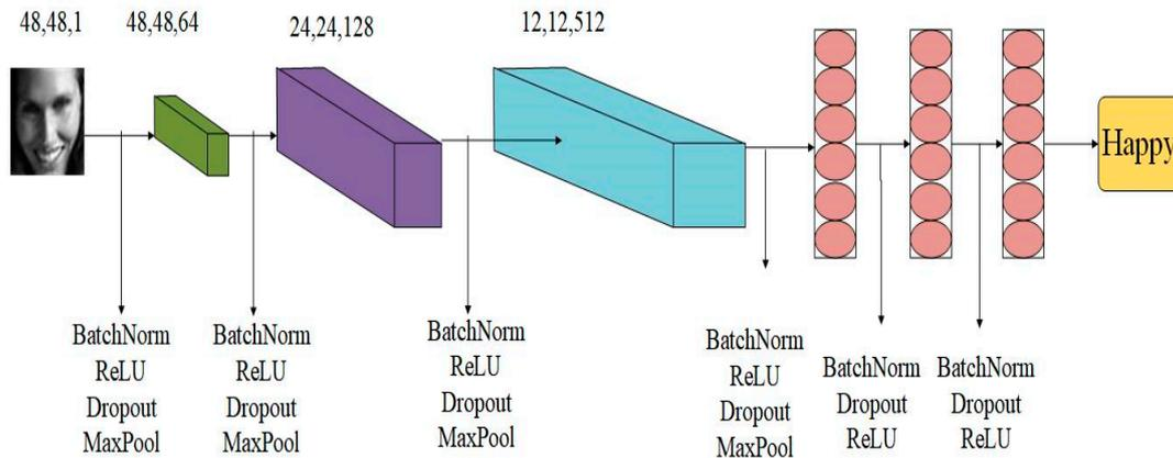
**Figure 5.** The architecture of CNN (Convolutional Neural Networks) is as follows: four convolution layers and two full connection layers.
