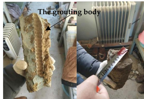
Figure 12. Glass fiber bolt grouting body.
