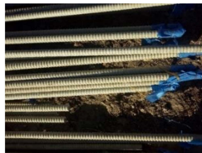
Figure 9. Glass fiber anchor.
