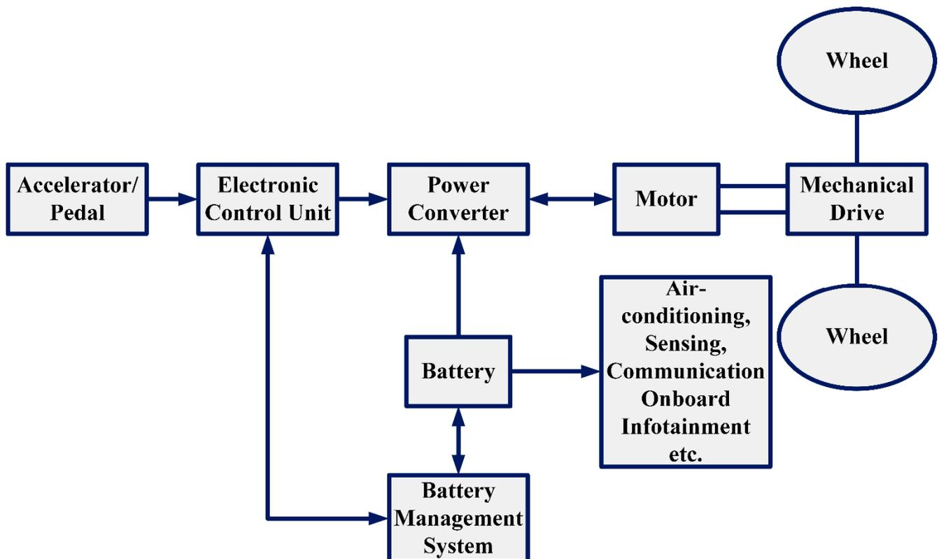
Figure 5. BMS operation inside Electric Vehicle (EV).
