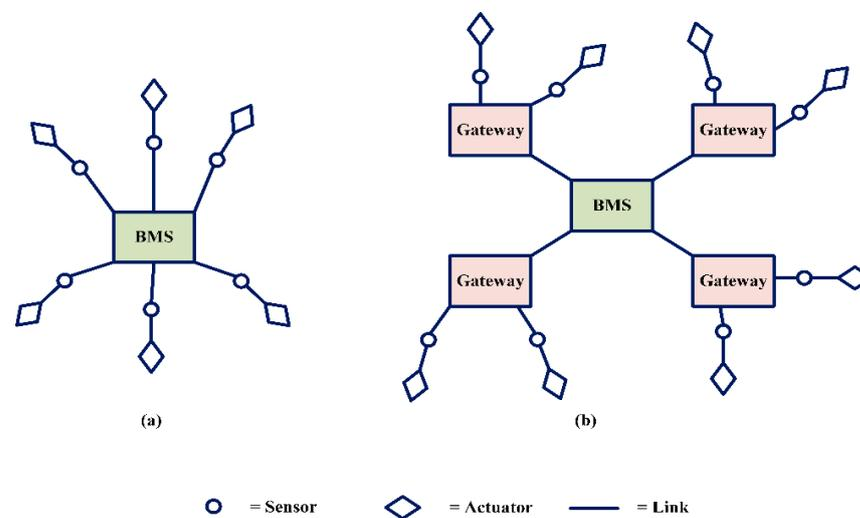
Figure 2. BMS implementation topology: (a) centralized, (b) distributed.
