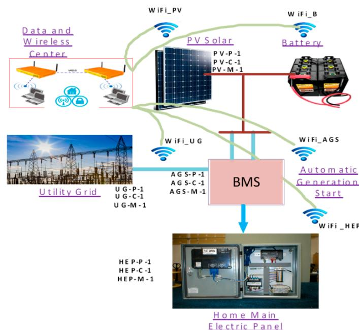
Figure 1. Battery Management System (BMS) connections and integrations [5].
