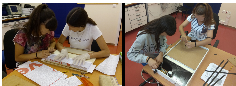
Figure 3. Students working on the construction of the \mu Cosmics detector unit. (Left) tiles are placed inside the wooden frame and wrapped with reflective paper. (Right) students attach the wooden frame inside the plastic box.
